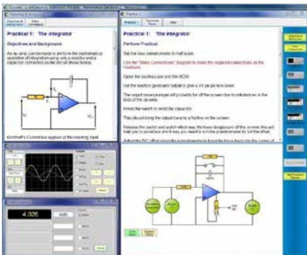
Screen showing the Feedback interactive ESPIAL software, enabling the student to learn the principles of the subject and then implement practical experiments using on-screen instruments.
